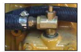
Double o-ring protection provides over 20,000 cycles without leakage!
