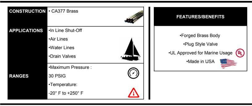
THE M670 SERIES Marine Fuel Valve is approved for use on Motor Craft Fuel Lines and is standard with a pointer lever and an internal 90° turn stop mechanism to assure positive location of the Off and On positions. Corrosion proofed internal construction assures maximum salt atmosphere protection. Port hole is 1/4" (.250) diameter.
